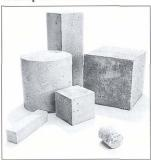
The PROCEQ conversion curve for a concrete age of 14 to 56 days has been defined with  $200 \times 200 \times 200$  mm test specimens. If the strength is defined on specimens of different dimensions, the strength determined from the curve is to be multiplied by the shape factor  $\alpha$ s. The relevant shape factor is to be obtained from the standards. For cubes of  $150 \times 150 \times 150 \, \text{mm}$ ,  $\alpha s = 1.05$ , for cylinders dia. 6" x 12",  $\alpha s = 0.85$ .
