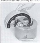
The testing anvil must be placed or a rigid and smooth surface (stone floor). The contact surfaces of anvil and hammer head must be cleaned. The SCHMIDT hammer for construction materials must reach the calibration value stated for the corresponding type on the anvil. If this is not the case, the unit must be overhauled by a service centre. The hammer (B) and its brake track in the housing should always
