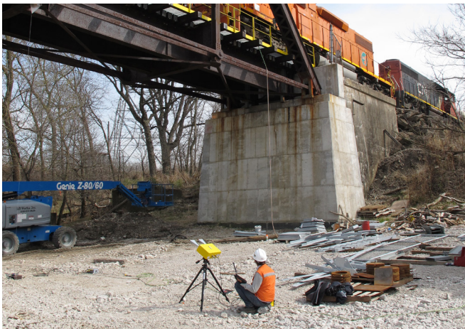
IBIS-FS monitoring an iron bridge
